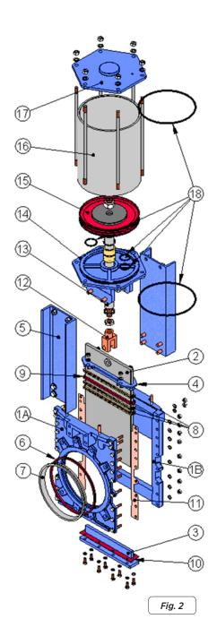
The yoke has a compact design with the bronze actuator nut protected in a sealed and lubricated box. This makes it possible to move the valve with a key, even without the handwheel (in other manufacturers' products this is not possible).
